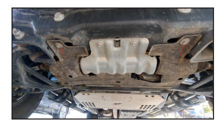
■1. Remove front factory felt liners and plates. Keep OEM bolts as indicated by arrows for later use.
