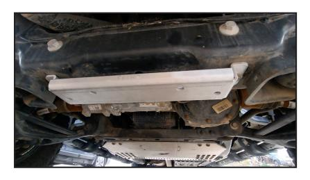
■3. Install middle bracket to front crossmember. Orient bracket as shown. Reuse OEM bolts to fasten to frame. Torque down to \*\*ft-lbs..
