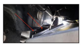
9. Middle bracket nuts can be reached and tightened from the side.
