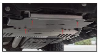
■5. Fitment: install flat plate loosely using OEM bolts (x2) in the rear and provided nut and bolt at the front (bracket side).
