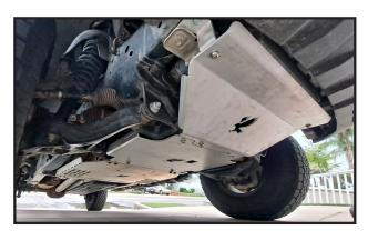
■11. Torque down all nuts and recheck torque values after first 100 miles and every 500 miles after that.
