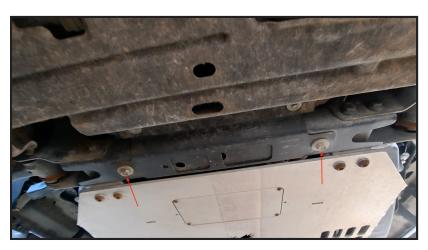
2. If your F-150 is not FX4 equipped, remove the black crossmember bracket that attaches the felt liners to the frame. Keep OEM bolts as indicated by arrows for later use.
