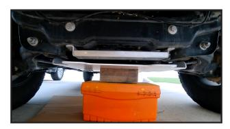
4. Elevate the flat plate to cover front diff/steering rack.
