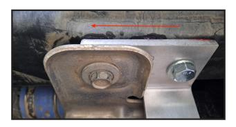
■7. Slide front plate brackets between intercooler bracket and frame as shown. Use provided hex bolt to fasten into provided U-nut.
