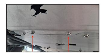
8. Install front skid using provided nuts & bolts. 2 rear (bracket side) and 2 front (intercooler side).
