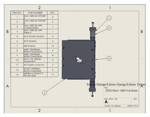
NOTE: Riv nuts are pre-installed and will not be in hardware kit.
