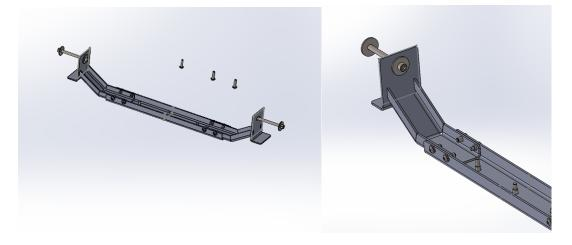
3. While it is possible to assemble the crossmember then install it, we have found it easier to loosely install the crossmember side pieces on the frame and then install the center piece.
