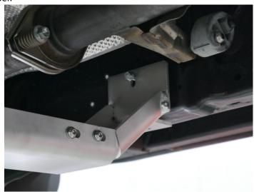
3. There will be an empty threaded hole on the passenger side frame rail across from the driver side bracket. You will install the other transfer case crossmember bracket on this bolt using the included M8x35mm bolt. Leave the bracket loose to allow installation of the center crossmember.
