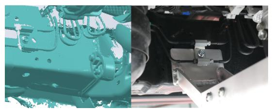
2. Locate the 12mm bolt on the driver side frame rail behind the transfer case cross member. Remove bolt. The bracket will pull away from the frame slightly. This will be needed in order to install the transfer case crossmember behind it. The transfer case crossmember will go between the line bracket and the frame. Use care not to damage the lines. You will replace the OEM bolt with a M8x35mm bolt included in the kit. Leave the bracket loose to allow installation of the center crossmember.
