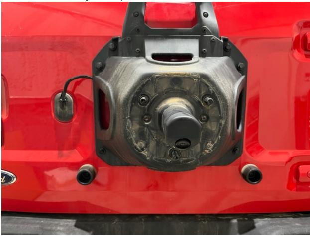
3. Remove factory spare tire and spare tire holder. Note that the backup camera and rear brake light connections are inside the driver side plastic cover you removed in the previous step. Unhook these connections first and pop out the rubber grommet from the inside. Now remove
