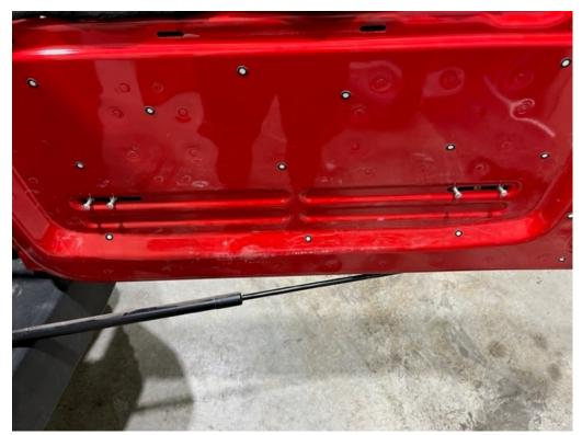
6. Once nut plate B is inside the door start the 4 M5x16mm button head bolts with washers in it. A magnetic telescoping tool may help line up the riv nuts. If you drop the nut plate you can use the magnetic pick-up tool to retrieve it. This step takes some patience to complete.
