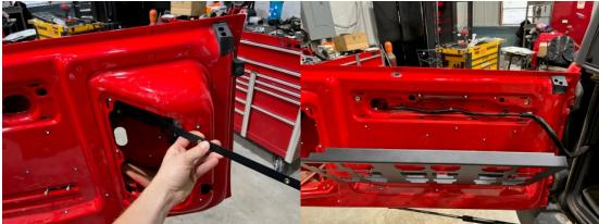
7. Obtain Nut plate A. Proper orientation will be as shown in photo above. Please note that on the passenger side where the door hinge is, the interior compartment shrinks. When inserting nut plate A, it is important to get Nut plate A forward of the protrusion to get it inserted all the way inside of the door. This may take a couple of attempts to get in. Remain persistent and you will succeed! You can secure the Nut plate in place with 2 M5 button head bolts.
