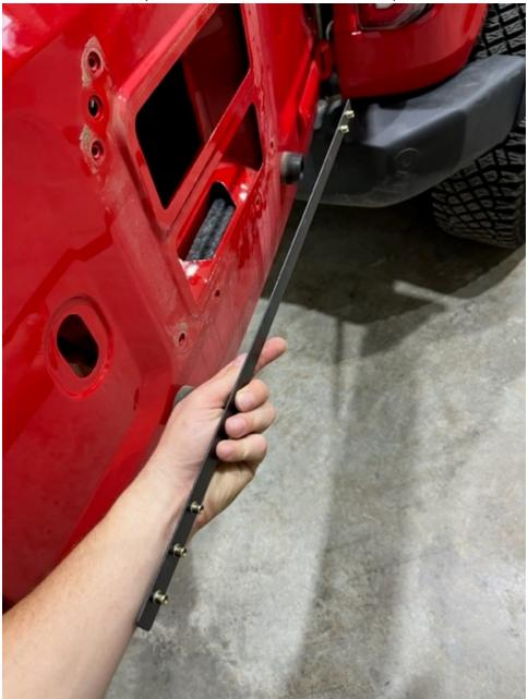
5. Find Nut plate B as shown in diagram above. Inside the bottom vent hole there is a trapezoidal hole with some insulation material inside. Nut plate B will feed inside this hole. The protrusion side of the nut plates will face towards the rear of the Bronco. Use care when you are fishing the nut plate inside the bronco that you do not damage the paint on the bronco or the nut plate.
