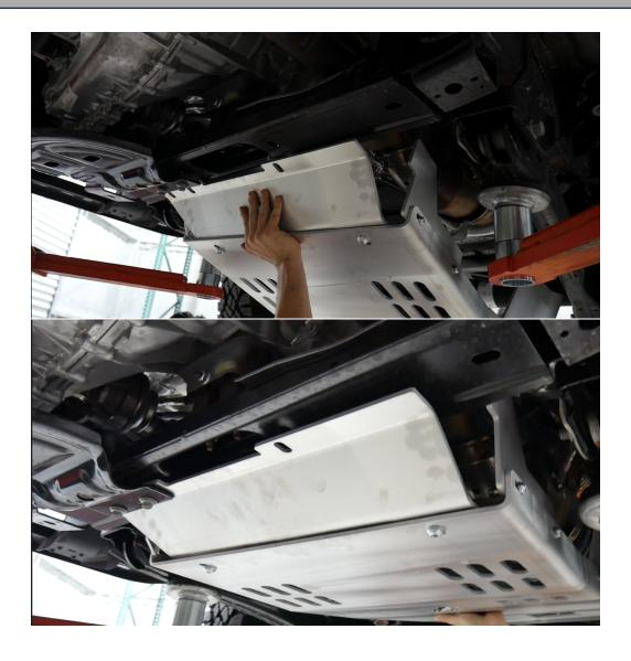
5. Pick up plate and install the rear portion between the transfer case skid plate and the frame. Ensure the bolts are still threaded enough to help hold the weight.
