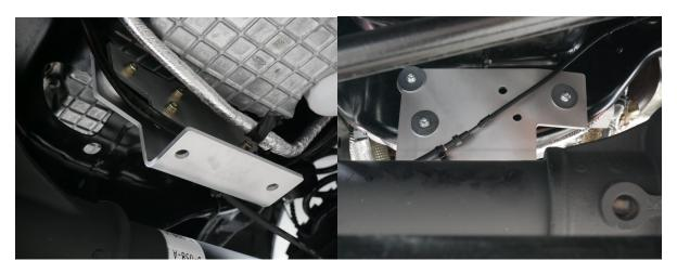
2. Install F-250 4G TM Mount A. This is figure one on the photos above. This plate will mount to the front of the engine crossmember. Please note that 2020-2023 and some 2023+ trucks will have different mounting hole configurations, so not all holes will be used.
