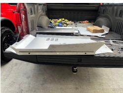
5. Install passenger side wing on transmission plate as shown. The wing will bend out from the plate, and will install on the inside of the flange on the transmission plate. You will use 3 M8x25mm button head bolts. 6 M8 washers and 3 M8 nylon lock nuts. Allen head size is 5mm.
