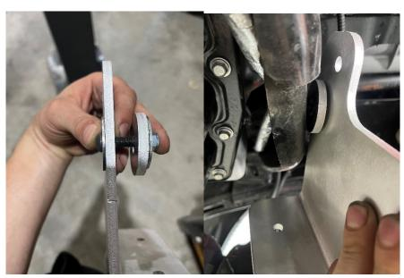
2. Correct install will have the spacer between the front mount and truck frame. Washers will go on either end.
