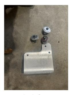
1. Gather the front mount, 3- ¼" spacers, M8x35mm Bolts, 1.5" fender washers and M8 nylon lock nuts to install.
