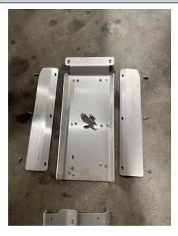
3. Install wings to the DPF Plate using the M8x25mm hardware. Wings will secure to the inside of the vertical flanges and bend outwards. Away from the center of the DPF Plate.
