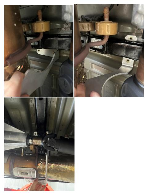
2. Install rear bracket up around upper cross member. It is easiest to lift and twist the bracket up into position. There will be a lower bracket that sandwiches the cross member. Use the 2 M8x80mm screws to secure.
