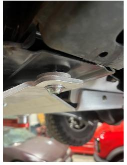
4. At this point you can lift the front DPF plate into positions. It is recommended you secure the front with the two M12 bolts, before securing it to the rear bracket. Allowing the weight of the plate to hang on the rear bracket could slightly bend the bracket. The
