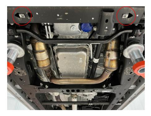
If OEM Engine skid plates are installed, you will need to loosen the rear of the engine skid plate. There will be two M8 spring clips. You can replace the factory OEM bolts with the included M8x40mm button head bolts. The transmission skid plate will slide between OEM skid plate and the factory frame.
