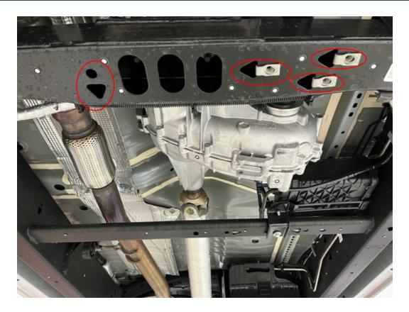
4. Install included M10x1.5mm spring clip on the hole to the left shown above. At this point you can install the 4 M10x50mm button head bolts into the rear of the transmission skid plate. These will go into the factory M10 spring clips. If you are installing with a Talons Garage Transfer Case skid plate you will want to install the Transfer case skid at this point with the Transmission Plate. The Transfer case skid will sandwich between the transmission plate and the frame of the truck.
