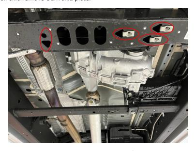
Install included M10x1.5mm spring clip in hole on the left in photo shown above. You can now install the Talons Garage Transfer Case skid plate into the 4 spring clips using the included M10x50mm bolts.
