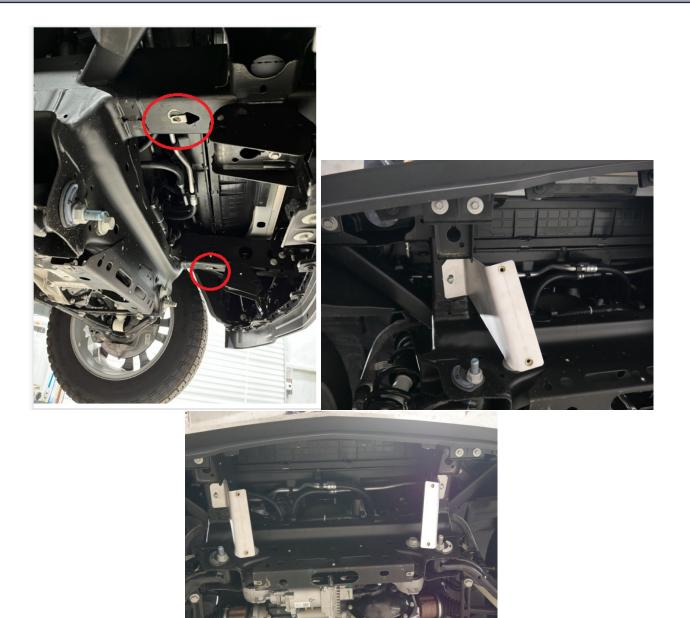
3. Start by installing your C1500 4G ENG BKT, item 2, Above. These brackets will be mirrored. Install at the top using a M8x40mm button head bolt. Leave these a little lose for the next step.
