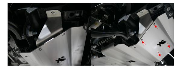
4. Lift the C1500 4G ENG Plate A up to the C1500 4G ENG BKT. You will use 4 M8x40mm button head bolts to secure the plate to the brackets.
