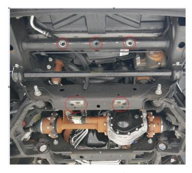
2. Grab C2500 4G ENG Plate A. This plate will replace the factory plastic skid. The front skid will mount in the 5 circled holes using the included M10 button head bolts. Leave bolts loose to install C2500 4G ENG Plate B. Note: our M10 button head bolts will use either a 6mm or 5.5 mm Allen bit depending on the brand. Ensure you use the correct bit to avoid stripping bolts.
