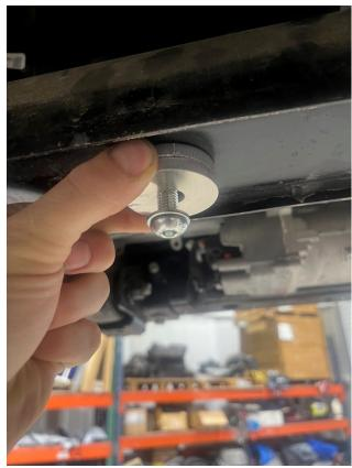
3. Spacers will go between the transmission plate and the frame. When installing at Talons we will gently guide the plate on the edge of the spacer, use the front of the plate to lift it up then slide the plate onto the bolts.
