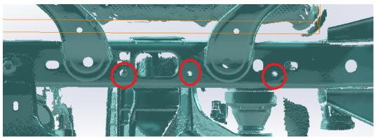
5. Note holes used to install rear of transmission skid. The two holes to the right are threaded. The hole on the left will require install of a nut clip.
