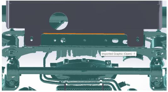
Install transmission skid plate front bolts, spacers and washers. On the crossmember ahead of the transmission there are 5 threaded holes. The transmission plate will use the 3 center holes. You will use one 10mmx40mm bolt, two ½" spacers and one 10mm washer on each hole. The outer two holes will be used either by the talons garage front plate, or the OEM factory front plate.
