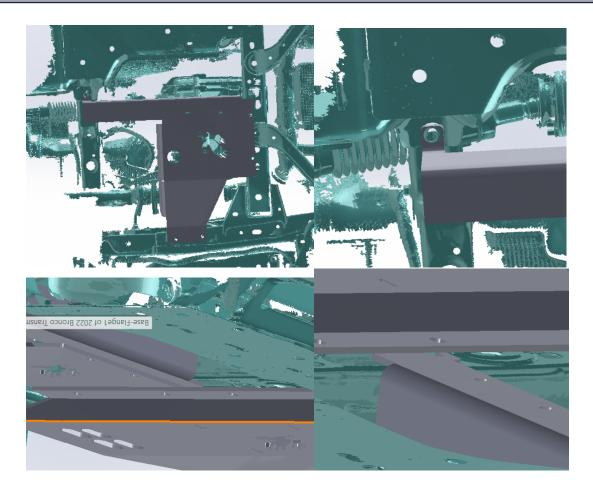
3. Ensuring fuel tank is properly supported, remove the fuel tank skid or strap bolt to allow install of transfer case cross member. Install Transfer Case Cross member. Transfer Case Brace will install to this bolt and slide above the transmission plate. CAUTION: If fuel tank is not property secured prior to removing the bolt, fuel tank may fall on you, which may result in death. Proper care is required to support fuel tank.
