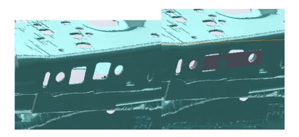
4. Slide riv nut plate into one of the rectangular holes. Align the riv nuts with the circular holes shown above.
