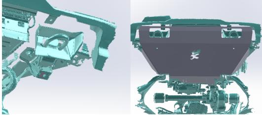
3. Mount Front Skid Plate to front mount, and to OEM mount points on intercooler Brackets. Having a helper to hold the plate up while you start the bolts helps. I found holding it through the eagle cutout and getting either the top or bottom bolts started helps.
