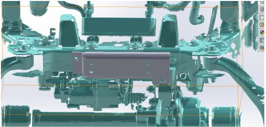
2. Mount Front Plate Main mount to frame using 2 M10x40mm button head bolts.
