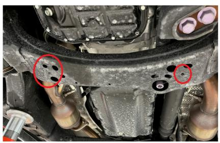
4. Locate the two M8 pre threaded holes. Clean out holes to ensure that the included M8 bolts will thread in easily.
