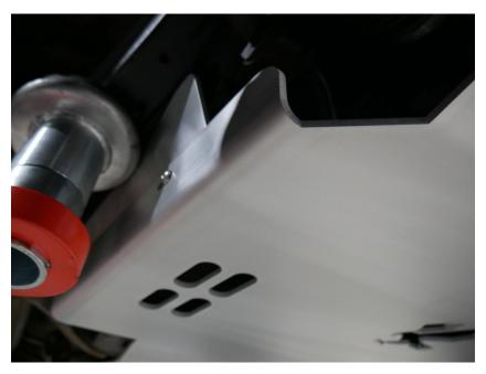
2. Install TM Winglet on passenger side flange of transmission plate. The winglet will bend towards the outside of the plate.
