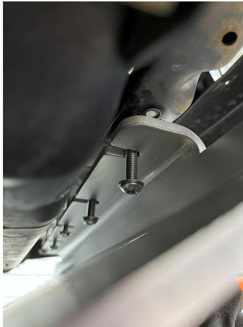
4. Obtain the 4Runner Engine Plate A. This plate will slide onto the bolts started into the cross member. You can carefully hang the plate there but be careful as it can fall and hit you on the head.
