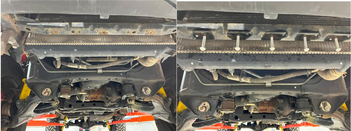
3. Locate the 5 pre threaded holes on the cross member directly in front of the radiator. The design of this skid plate allows you to use all five holes. Due to the age and potential for some of the threaded holes to be unserviceable to recommend at least using two holes on either end of this skid plate. Start the M8x40mm bolts with a M8 washer on each of the holes.
