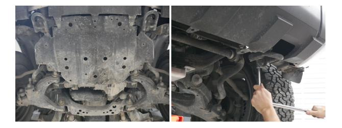
1. Remove factory front skid plate and braces. Loosen tow hooks leaving front bolt in place and removing the rear bolts. Save bolts.
