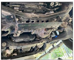
2. Install front skid plate bracket to the 3 M8 threaded holes on the engine cross member. Leave bracket loose to allow for alignment.
