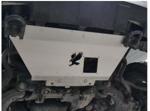
3. Install front skid plate. Front of skid plate will slide under the factory tow hooks. Rear of skid plate will install to mount with M12 Allen head bolts. Bumper tabs can sandwich between frame and skid plate to hold them in place.
