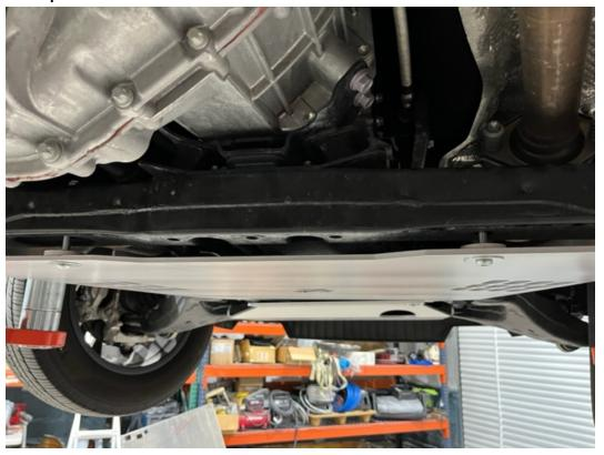
3. If Talons Garage Transmission skid plate is already installed, or you are installing the transfer case skid plate with the transmission plate you will want to remove the rear bolts on the transmission plate and loosen the front ones to allow the rear of the plate to hang down. At this point you will want to locate the two ½" thick round spacers. These
