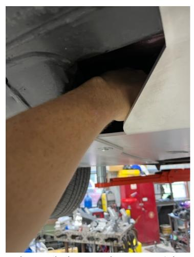
6. After getting the M8 bolt started, you can tighten all the bolts. Use 10 Ft Pound of torque on all the bolts. The nuts on the back end of the transmission plate/Front of transfer case plate can be accessed from the rear side of the truck. Shown above is how I accessed the nuts. I used a open ended wrench and reached up into the area between the
