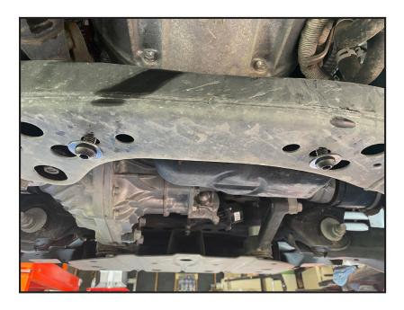
■2. Install the M12x100mm bolts with the nuts up into the holes from step one. You will use the larger washer on the top. Leave these bolts hanging.
