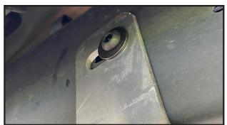
the rear of the plate. The M8x100mm bolts will go through these holes, into the frame. Install the large 3/8" washer on this bolt, with the nut above the frame. If you are installing a transfer case plate with this, be sure to put the 3x3" spacer between the transmission plate and the
