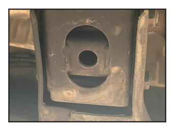
3. Slide the front of the catalytic converter protection plate over these bolts. It should hold the plate in place.
