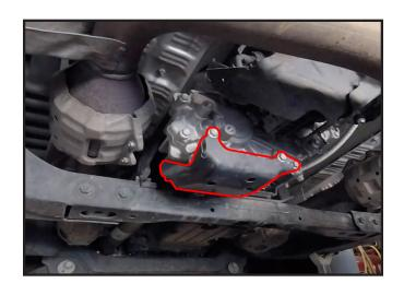
■3. If this is a 4x4 truck, remove factory transfer case shield.
