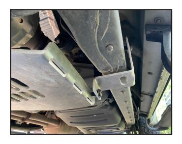
■5. Attach Z brackets to ½" holes on the rear of the transfer case plate.
