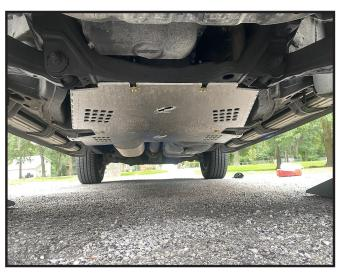
•• 6. At this point, if you are installing the transfer case plate with the transmission plate, tighten all bolts starting from the front bolt and working your way forward.
