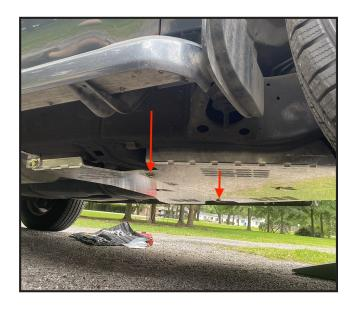
■1. If Transmission rear bolts are not loose from install, loosen transmission rear bolts and install the square spacers above the transmission plate.
