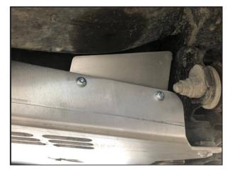
2. Install the two winglets on the sides of the plate like shown above. Mount using 4 M8 x 25 mm bolts, 8 small washers, and 4 nuts.
