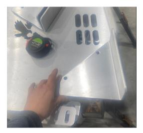
1. Install the included wings on the transmission plate. These wings will go on the inside of the plate and will bolt in with the included M8 x 25mm bolts. Use a smaller M8 washer under each bolt head and a larger 1-inch washer under each nut.
