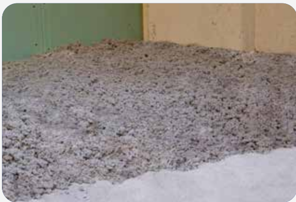
THERMOFLOC floor filling as cellulose insulation not resistant to compression
