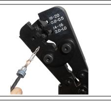
3 Insert the terminal and seal into the matching cavity until it is fully seated within the mounting block.
