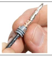
5 Once the jaws release, remove the crimped terminal and seal from the jaws.
