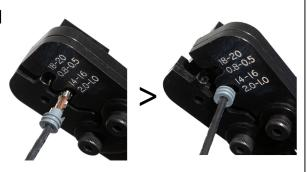
6 Gently pull on the terminal to ensure the crimps are secure.
