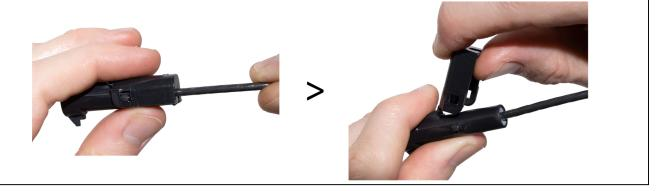
2 Center the tool's metal barrel around the now exposed terminal and press it into the open cavity until it stops.
