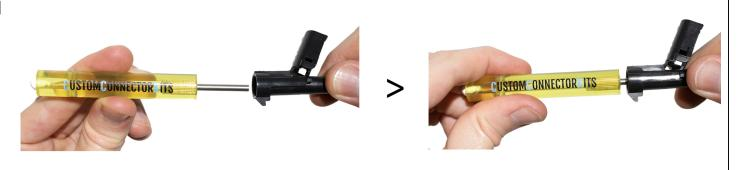
3 Gently pull the wire from the back of the conenctor to release the terminal from its locked position. The tool can be removed from the cavity now.
