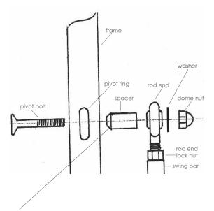
Note: Ensure that tapered end of spacer bush fits to the ring on the frame or damage can occur.
