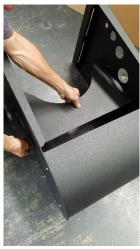
Step 4: fit gusset with 4 bolts, do not tighten.
