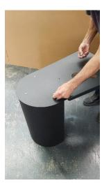
Step 2: fit side panel to barrel, using 3 bolts supplied. Do not tighten at this point.
