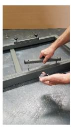
Step 5: remove clamp bars from main frame.
