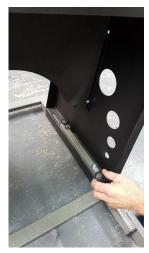
Step 7: re-fit clamp bars, washers and hand nut. Now tighten all of the bolts in the barrel and gusset.
