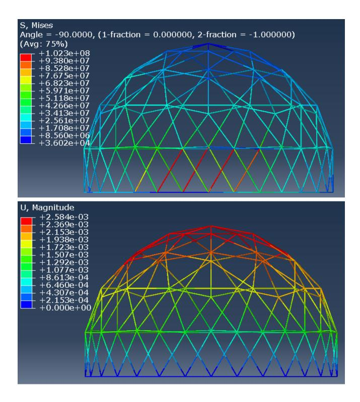
From the above figures, we know maximum Von Mises stress and maximum displacement happens in the load case 4 (1.4W+0.5S).
