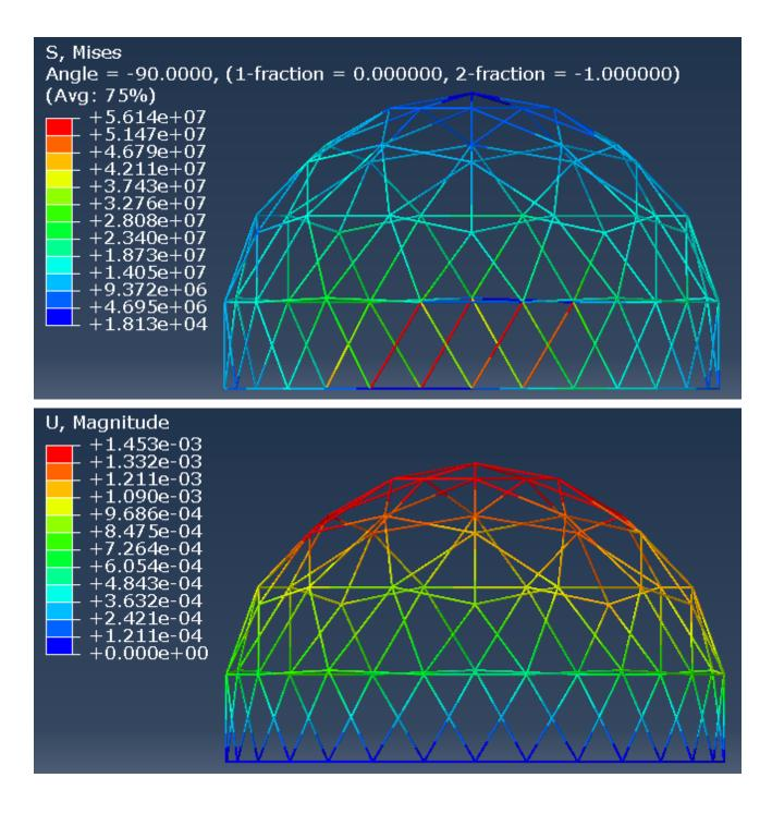
From the above figures, we can know maximum Von Mises stress and maximum displacement happens in the load case 3(1.5 S+0.4W).
