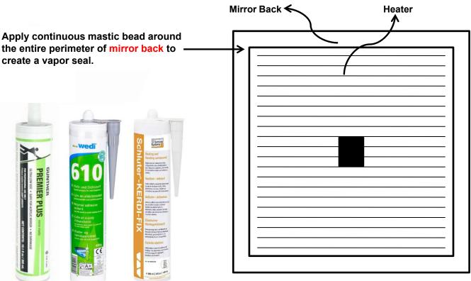
Apply adhesive on the open mirror surface and to heater for mounting to wall.
