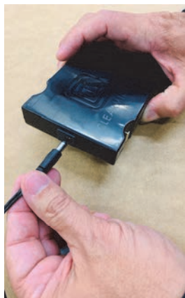
Figure 6. Charging the battery and inserting in mirror.
