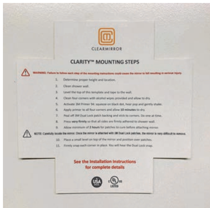
Figure 1. Determine mounting location.
