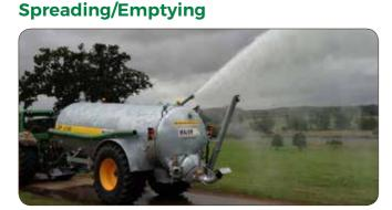
Centre mounted or rear mounted in conjunction with a garda pump fitted with stone trap as standard
