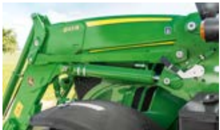
1 Underslung levelling link The ingenious geometry of our front loader linkage brings several practical advantages. Because the levelling link is underslung it cannot impair the operator's view. It also conveys more power along the loader shafts, provides easy access for servicing and allows greater steering angles.
