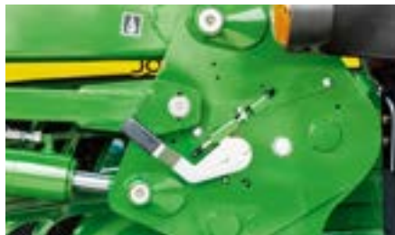
2 Automatic mast latch Mounting our front loaders could not be quicker, safer or more convenient thanks to the built-in automatic mast latch. You need to leave the cab only once. Separating tractor and loader is just as easy.
