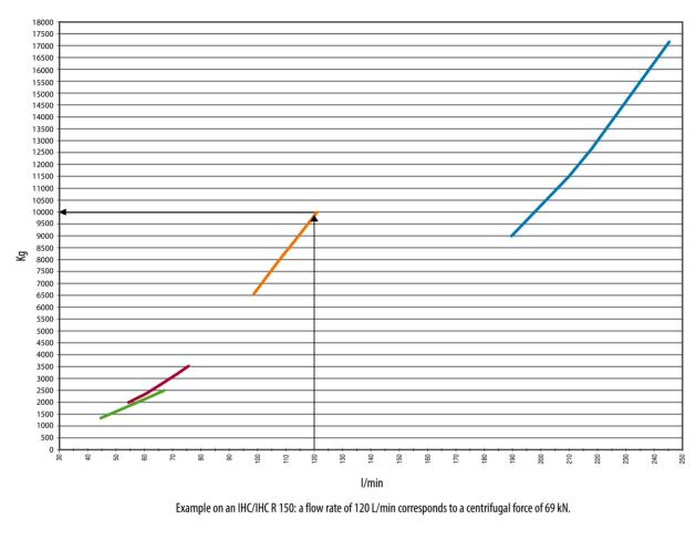
\_\_\_\_\_ IHC/IHC R 50 \_\_\_\_\_ IHC/IHC R 70/75 \_\_\_\_\_ IHC/IHC R 150 \_\_\_\_\_ IHC/IHC R 250
