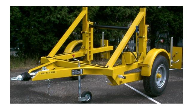
Our robust Trailers present an ideal means of transporting Cable Drums from contract to contract or around your job site. With a built-in suspension system, the Drum sits tightly on a central spindle, allowing conductor stringing operations when the integral parking brake is engaged.
