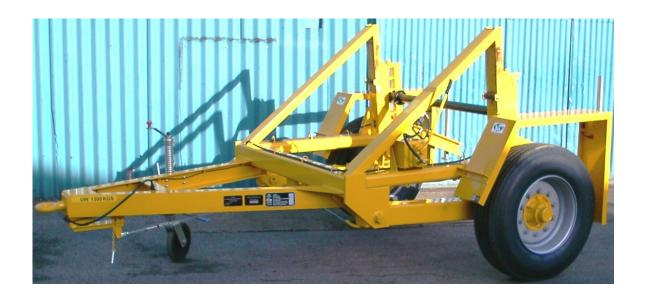
Our robust Trailers present an ideal means of transporting Cable Drums from contract to contract or around your job site. With a built-in suspension system, the Drum sits tightly on a central spindle, allowing conductor stringing operations when the integral parking brake is engaged.
