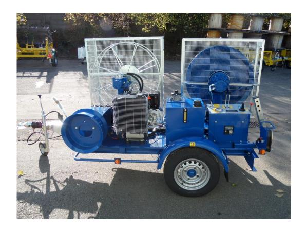
The Assist Winch can be used for the installation of fibre optic cable, sub duct and also for pulling the bond back through the duct or trench. For added safety they are fitted with cages covering the Capstan and the storage reel.
