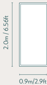
SINGLE DOOR FRAME Inside 1.92m/6.3ft x 0.82m/2.69ft
