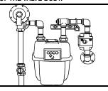
9. PROPER STABILIZATION OF THE VALVE INSTALLATION IS ESSENTIAL TO AVOID NUISANCE TRIPPING. TO STOP EXCESSIVE VIBRATION AND TO COMPLY WITH CODES, BRACE THE VALVE WITH THE LITTLE FIREFIGHTER GV-12 STABILIZER BRACKET.
