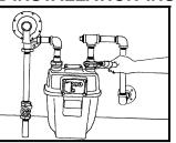
3. Remove the union from the house side of the meter with a pipe wrench and detach the union & tee from the pipe nipple.
