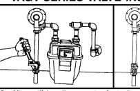
2. After notifying all occupants of affected structure that the gas will be shut off during the installation, shutoff all appliances and pilot light valves. Verify the gas in the house is off with the wet paper method from step #1, and then turn the wrench operated meter inlet valve off. Do not tamper with the
