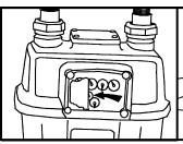
1. Before Starting, check to insure the meter is functioning properly by wetting a piece of paper and pasting it over the centerline of the hand of the 1/2-foot dial of the gas meter. Turn on a gas appliance and observe the motion of the hand after five (5) minutes. Notify the Gas Company if the meter is bypassed or defective.
