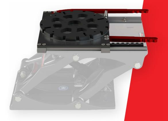
This Swivel Slide system has 5-inches of fore-aft travel and features premium track and cars for smooth operation. The 360-degree swivel has a positive lock that engages every 22.5° (16 positions).
