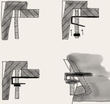
Immediately reintroduce the sink in the marked position. Next, put the anchor claps over the spiral that were set up previously and tighten the screw until it is held firmly
