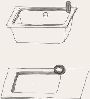
Complete the installation of the valve. For a perfect positioning, protect the sink tape laid 2 mm away from the joint. The countertop must also be protected with tape.
