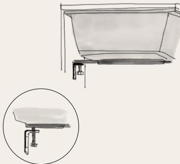
Fit the sink in its final position and put the anchor support over the framing square until the sink is held. Confirm the top part is in the desired position and adjust the anchor again if its necessary.
