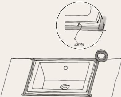
Fit the sink into the countertop, checking that there is no light showing through. Next, protect the sink with tape 2 mm away from the sink.
