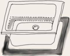
Check that the sink fits without interfering with the clamping zones and without any visible light showing through. To do this, use the sink over the hole or with the template given, only in those models that include it. Templates that are not included in the box can be downloaded from our web [www.poalgi.es/en](http://www.poalgi.es/en)
