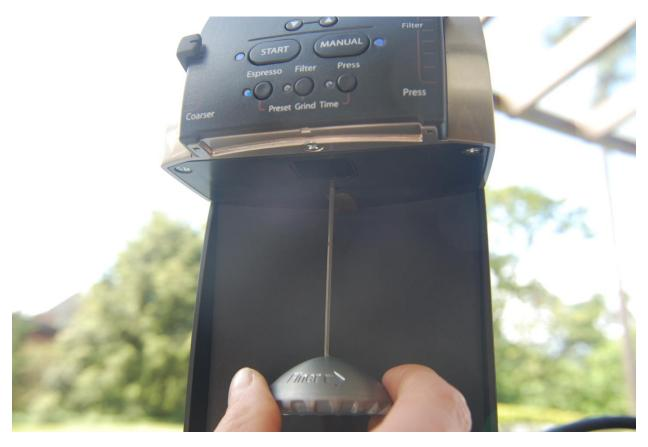
With the motor running, slowly twist the tool finer until you hear a change in noise. Turning the tool should require minimal force.
