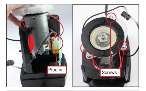
Secure the safety interlock switch onto it's posts.
