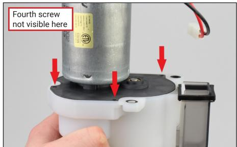
Install the gearbox/ motor assembly back into the chassis. Plug motor cable into board.
