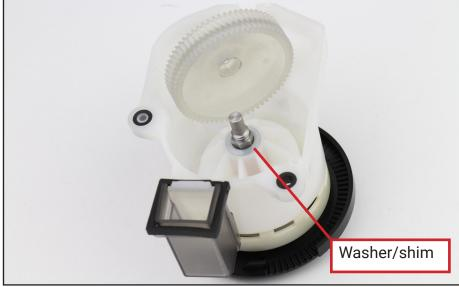
There will be several washers between the paddle wheel and gearbox housing. Remove the washers and paddle wheel. Keep them in a safe place separate from the drive gear/gearbox housing washers to avoid confusion.
