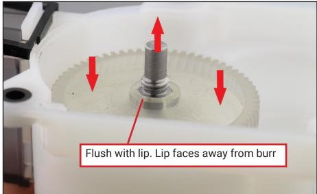
\*If having difficulty getting flush, make sure paddle wheel pegs are still indexed into cone burr. You can use your old cone burr as a block to help apply pressure with two hands to the drive gear if needed\*
