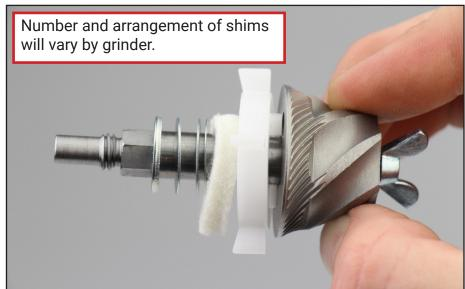
\*If the various shims were not kept separate, reference the GB2.0 guide for help re-arranging them\*
