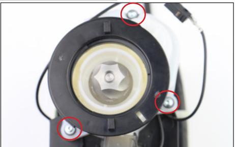
Lift the gearbox/motor assembly up and away from the chassis. Unplug the motor cable from the board.
