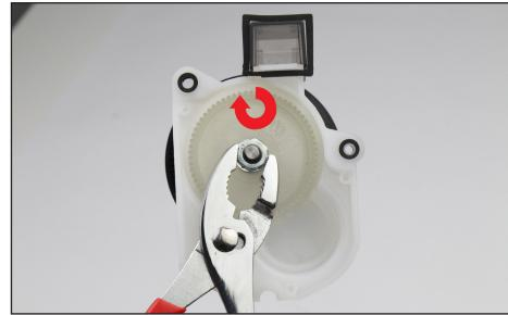
Attach the motor/motor plate to the gearbox. Tighten screws in a X pattern.
