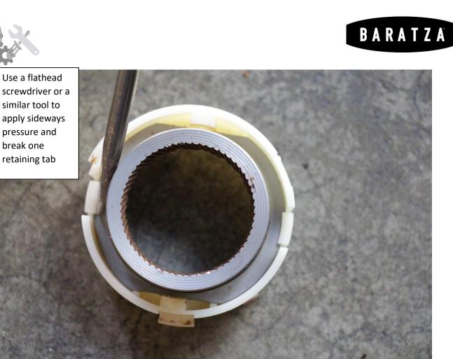
Once a retaining tab is broken, the metal will easily separate from the burr holder
