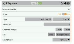
The external RF module can be powered on or off by software. The setup process is the same as that for the internal RF. External modules should be closed when not in use
