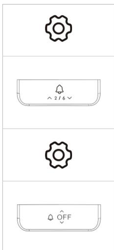
2.1 In the display height digital interface, press the right setting key
