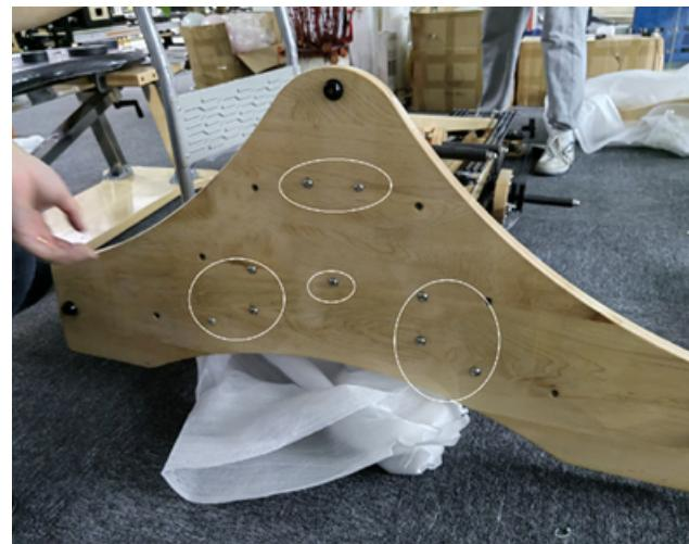
**Step 2:** Use 6 black long bolts to secure the support legs with the base board
