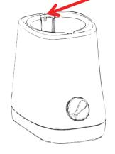
If you find that the water in kozii is rising and circulating, but not getting warm, this probably means kozii was run dry, and the safety thermostat has tripped. To reset it, do the following:
