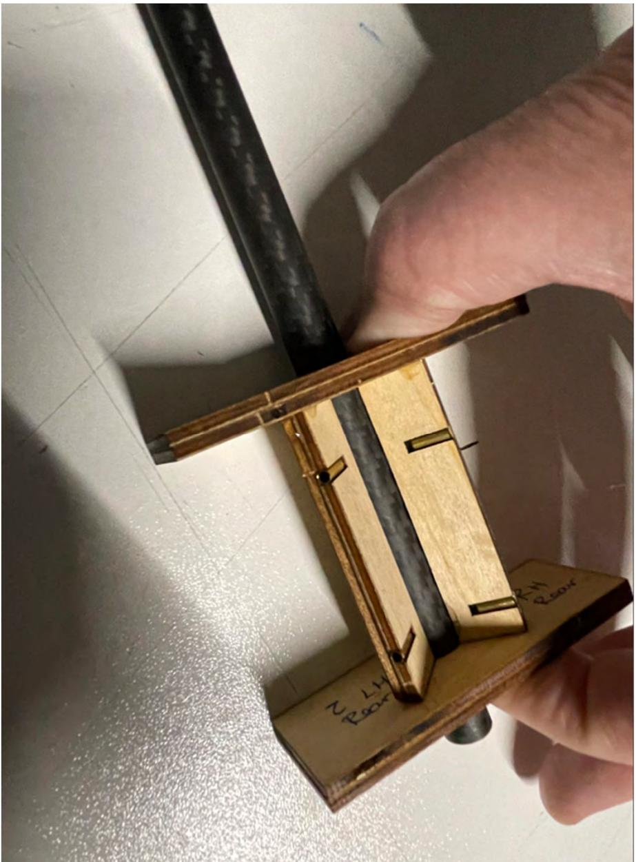
Unassembled the jig and apply thick CA (Superglue) at the interface of each of the 4 parts.
