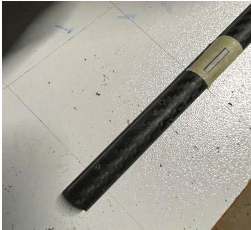
Remove the 2mm carbon locator rod and remove the boom from the v tail drill jig.
