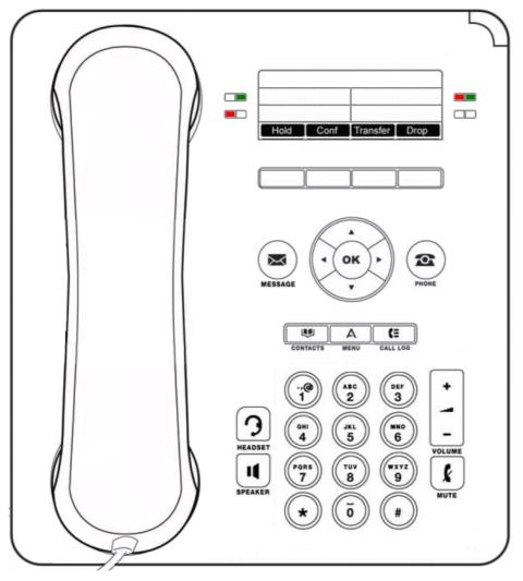
This phone supports 12 programmable call appearance/feature buttons. The labels for these buttons are visible on the main display and can be controlled by the adjacent buttons.
